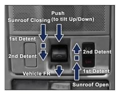
This switch is used to open, close, tilt up & tilt down the sunroof as and when required with switch intended operation.
