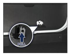
In case of electrical malfunction, you can unlock the tailgate from inside as per procedure given below:
