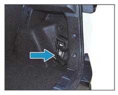
Remove the two Velcro as shown in figure and take out the puncture repair kit.
