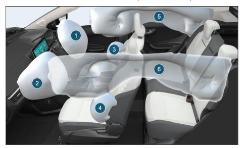
The SRS [Supplementary Restraint system] is designed to provide protection to occupants in case of collision or sudden impact, when crash is detected, the SRS airbag system deploys airbags to help reduce the risk of injury to the occupant. It works in conjunction with seat belts.
