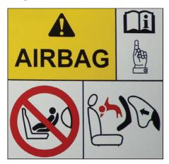
The Airbag Warning Symbol on sun visor reminds of the extreme hazards associated with the use of a rearward-facing child restraint on front passenger seat during airbag deployment. It does not mean that a child cannot occupy front passenger seat and use seat belt. Please refer CRS section for recommended seating position for children.
