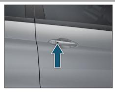
Press the door handle switch (DHS) provided on the driver door to lock/unlock all the four doors except Tail gate.
