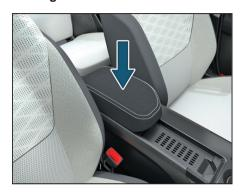
Stowage compartment is provided below the foldable arm rest for keeping cell phones, iPod's, chargers etc.
