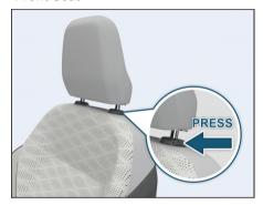
Adjust the head restraint so that it is as close to the head as possible and center of the head restraint supports the back of the head at eye level.
