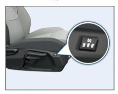
It has 3 ventilation adjustment in decreasing order and LED glows for each press. To Stop the ventilation long press the button for few seconds.
