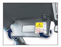
The sun visors can be pulled down to block the glare coming through the wind-shield. To block the glare from side windows, pull down the sun visor and release it from retainer. Swing the sun visor to the side.
