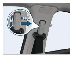
If height adjustment is provided in the seat belt, occupant can adjust it as per their comfort.
