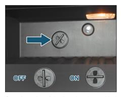
On selected models glove box is provided with a cooling facility. It cools the glove box only when the front A/C is ON. Shut OFF the vent by rotating the knob, whenever cooling is not required.
