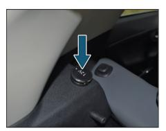
The power socket will work when the ignition switch is in the "ACC" or "ON" position.
