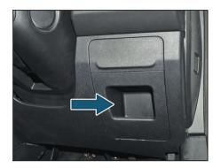
Stowage is provided on RH side of steering wheel for Coin, mobile and wallet.
