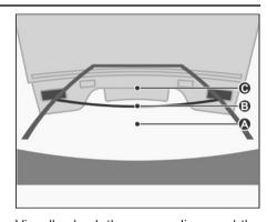
Visually check the surroundings and the area behind the vehicle. On the screen, it appears that a truck is parked at point B. However, in reality if you back up to point A, you will hit the truck. On the screen, it appears that A is closest and C is furthest away. However, in reality, the distance to A and C is the same, and B is further away from A and C.
