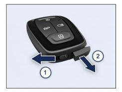
Slide the knob (1) to release the key. Pull the key blade (2) out.
